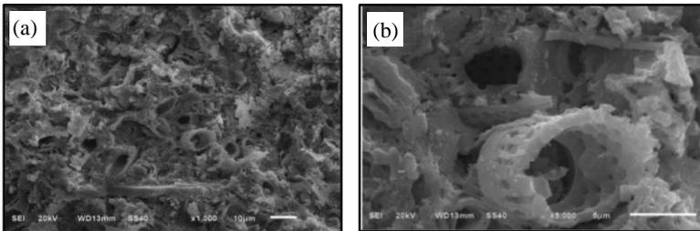
Figure 9. SEM images of fractured surfaces of SC12 (55C/45S-WOS) slip cast samples fired at 1050oC (a) x1000 (b) x5000 magnification
