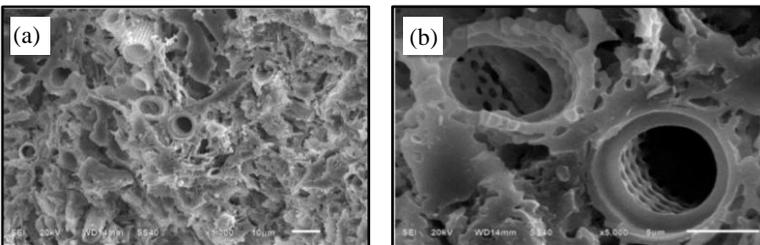
Figure 10. SEM images of fractured surfaces of SC12 (55C/45S-WOS) slip cast samples fired at 1150oC (a) x1000 (b) x5000 magnification
