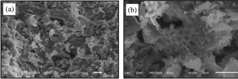
Figure 7. SEM images of fractured surfaces of SC6 (45C/55S-WCA) slip cast samples fired at 1050oC (a) x1000 (b) x5000 magnification
