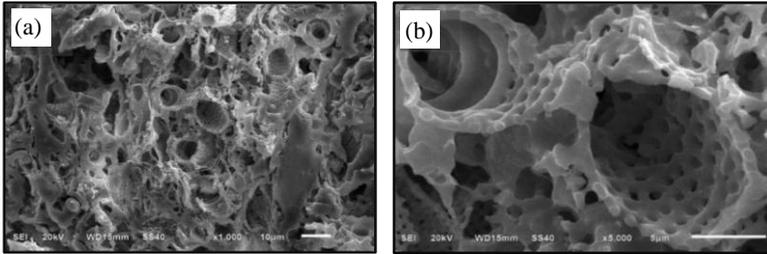
Figure 8. SEM images of fractured surfaces of SC6 (45C/55S-WCA) slip cast samples fired at 1150oC (a) x1000 (b) x5000 magnification
