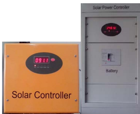
Figure 7. Solar ChargeController (left –TS96S60P& right –TS220S80P)
