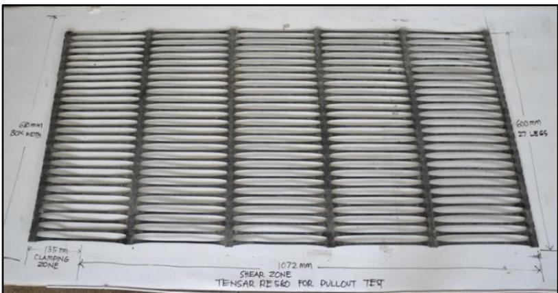
Figure 6. Tensar RE580 sample for the pullout tests
