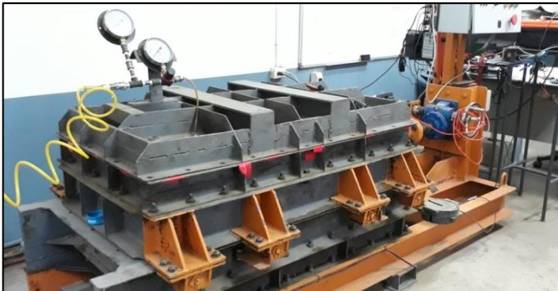
Figure 5. Large-scale direct shear box
