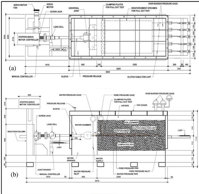
Figure 1. Plan (a) and section (b) of large-scale pullout box
