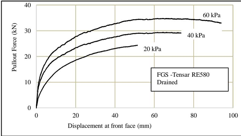
Figure 19. Load-displacement curve for FGS-Tensar RE580 under drained loading
