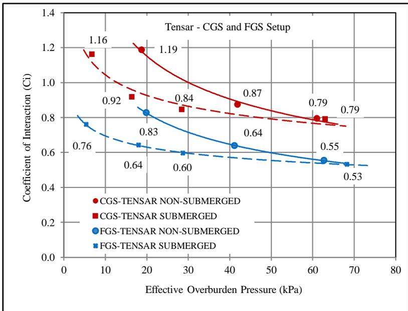
Figure 24. Coefficient of interaction curves for FGS and CGS interfaced with Tensar RE580
