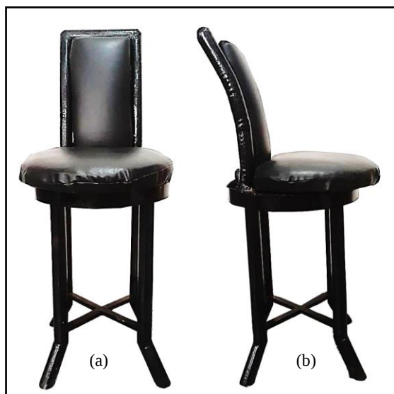
Figure 11. Fabricated IFaDes chair with backrest front (a) and side view (b)
