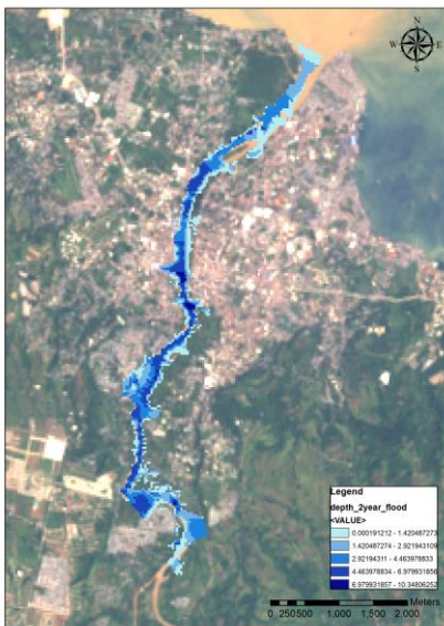
Figure 17. 2-year flood depth
