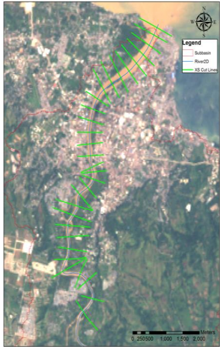
Figure 16. Cross-section cut lines for hydraulic model in HEC-RAS
