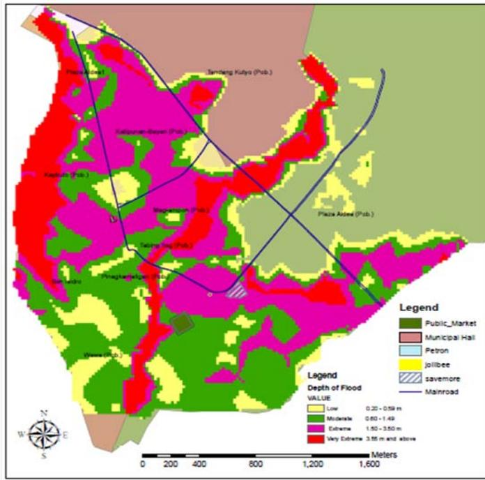
Figure 8. Simulated depths and extent of flooding using extreme rainfall data and the present land cover of the watershed
