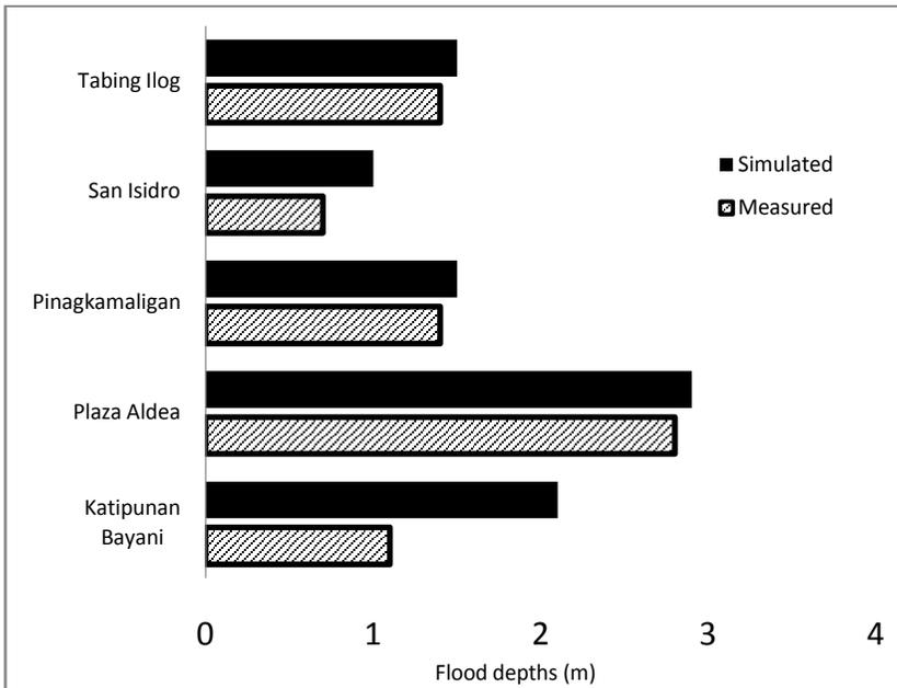
Figure 11. Simulated and measured flood depths during Typhoon Ondoy
