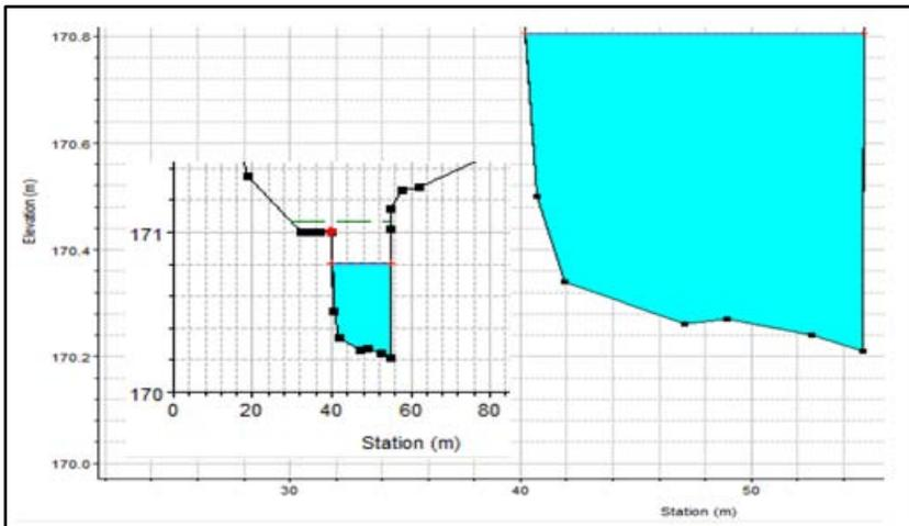
Figure 7. Simulated water depth in the middle of the river network using a peak discharge of 16.9  $\text{m}^3\text{s}^{-1}$
