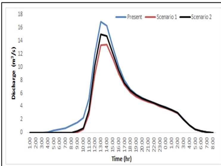
Figure 6. Simulated hydrographs of the middle river network using 80 mm total rainfall
