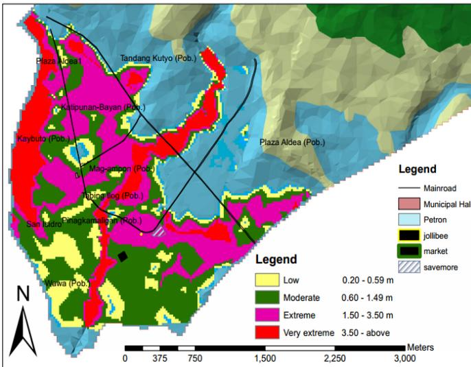
Figure 9. Simulated depths and extent of flooding using extreme rainfall data and the 1<sup>st</sup> land cover scenario of the watershed
