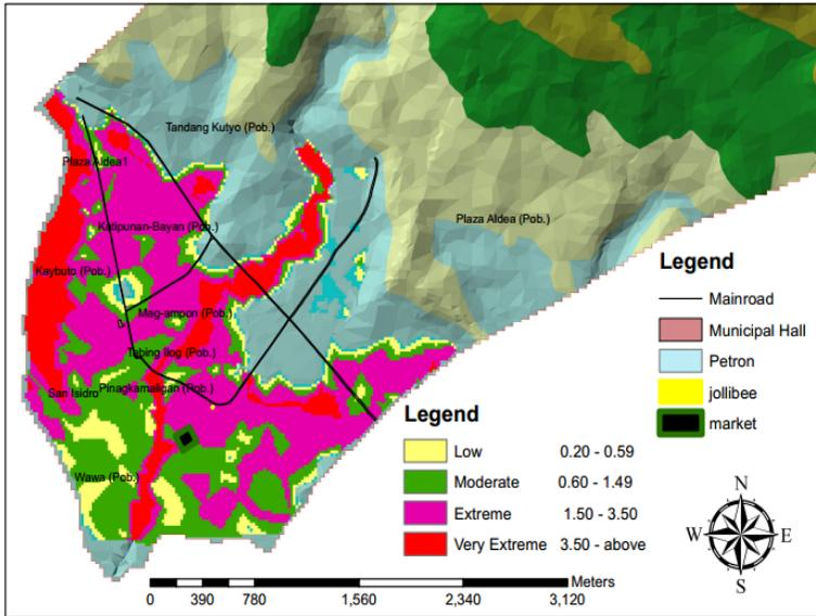
Figure 10. Simulated depths and extent of flooding using extreme rainfall data and the 2<sup>nd</sup> land cover scenario of the watershed
