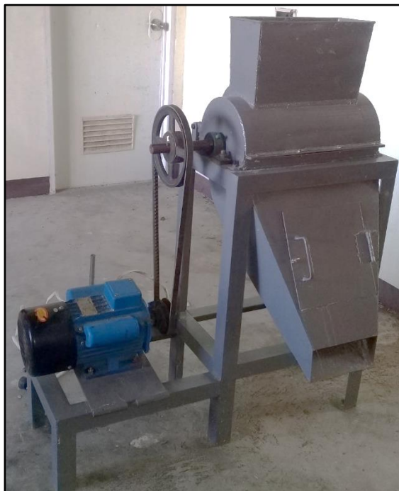
Figure 5. Actual view of the motor-operated cassava grater
