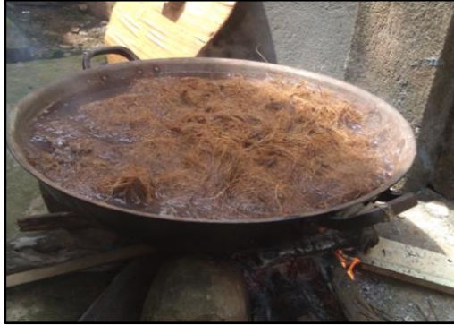
Figure 2. Boiling of coconut fiber for two hours
