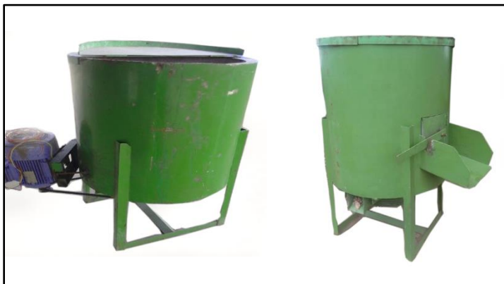
Figure 2. Actual appearance of the cassava peeling-and-washing machine
