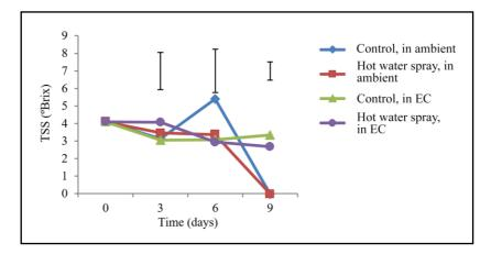
Figure 4. Effect of hot water spray treatment and storage in cabinet EC on the TSS of sweet pepper. Vertical bars indicate LSD value at  $p \le 0.05$ .
