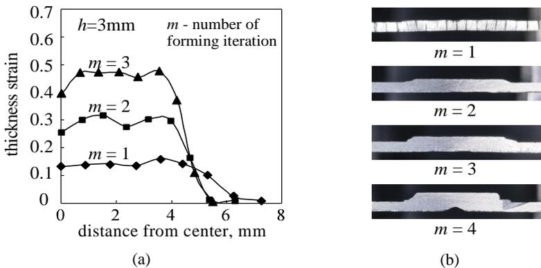
Figure 5. (a) Thickness strain distribution after a number of forming iteration,  $m$ , at a bead height of 3mm (beading die width = 6mm; compression die width = 10mm; Al-O;  $t = 1\text{mm}$ ). (b) Final shape of the specimen at several number of forming iteration,  $m$ .
