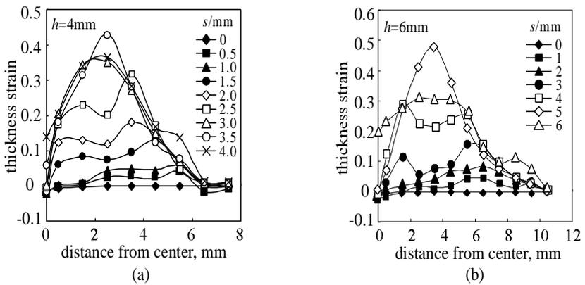
Figure 3. Thickness strain distribution at various compression strokes,  $s$ , utilizing (a) beading die width=6mm; compression die width=10mm (bead height=4mm) and (b) beading die width=12mm; compression die width=16mm (bead height=6mm).
