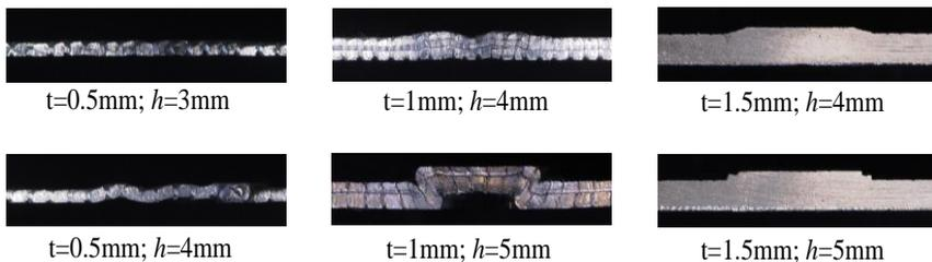
Figure 8. Final shape of the specimens at various sheet thickness and bead heights after compression with lubrication
