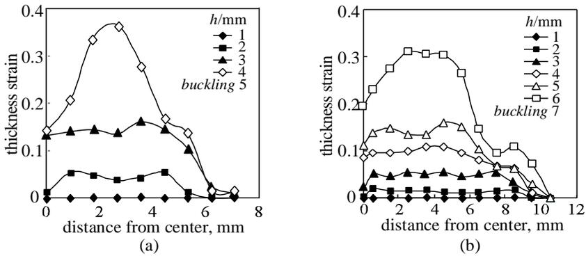
Figure 4. Thickness strain distribution at various bead heights,  $h$ , after compression utilizing (a) beading die width=6mm; compression die width=10mm (bead height=4mm) and (b) beading die width=12mm; compression die width=16mm (bead height=6mm).
