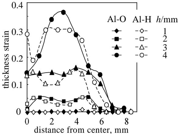
Figure 6. Effect of material type on the thickness strain distribution at different bead height,  $h$ , after compression. ( $t=1\text{mm}$ )
