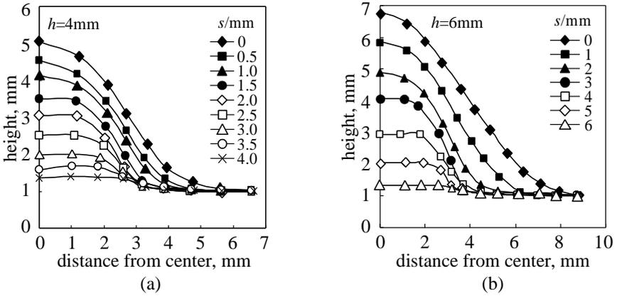
Figure 2. Deformation behavior of Al-O ( $t=1$ mm) at various compression strokes,  $s$ , utilizing (a) beading die width=6mm; compression die width=10mm (bead height=4mm) and (b) beading die width=12mm; compression die width=16mm (bead height=6mm).
