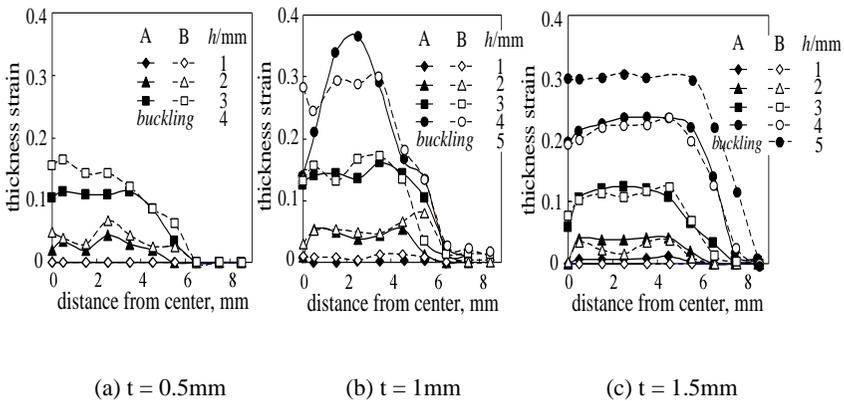
Figure 7. Effect of lubrication (A: no lubrication; B: with lubrication) on thickness strain distribution at various bead heights,  $h$ , after compression of Al-O with sheet thickness of (a)  $t=0.5\text{mm}$ ; (b)  $t=1\text{mm}$ ; and (c)  $t=1.5\text{mm}$ .
