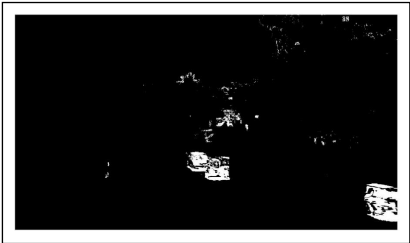
Figure 6. Frame subtracted to adaptive background
