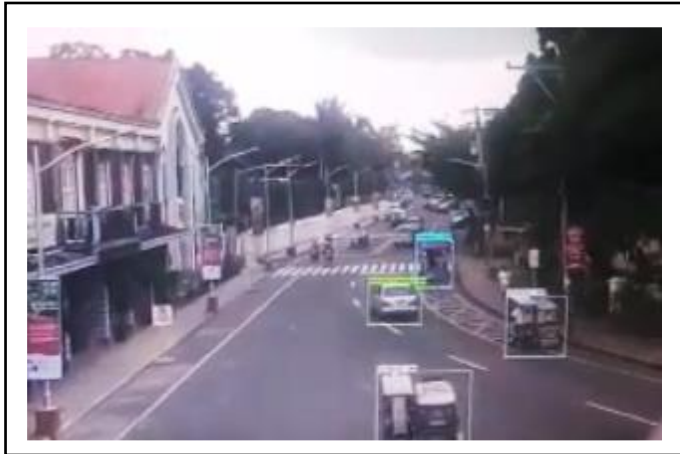
Figure 15. Vehicle detection with bounding boxes
