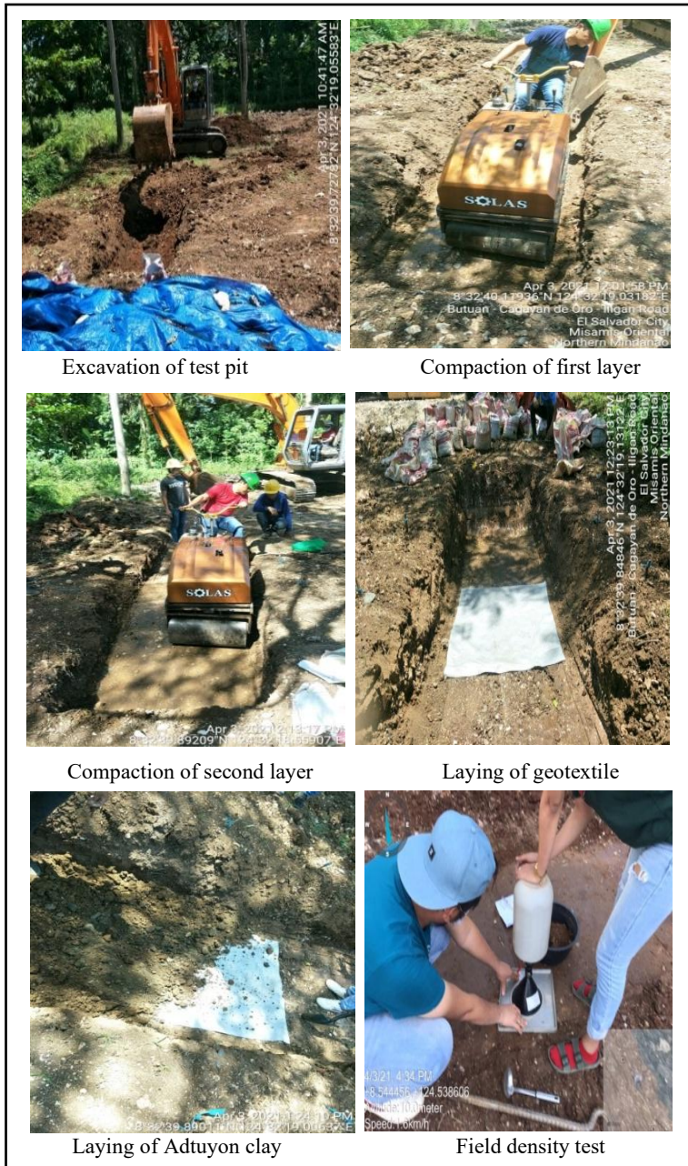
Figure 5. Sample preparation before the plate load test
