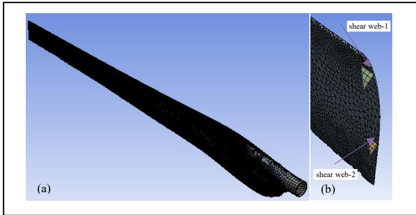
Figure 5. Meshing results on the model (case Alt-4) blade surface (a); and blade shear web (b)
