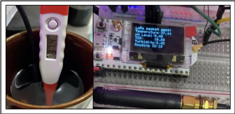
Figure 9. Temperature Reading of Purified Water 3 using a Digital Thermometer and Temperature Sensor
