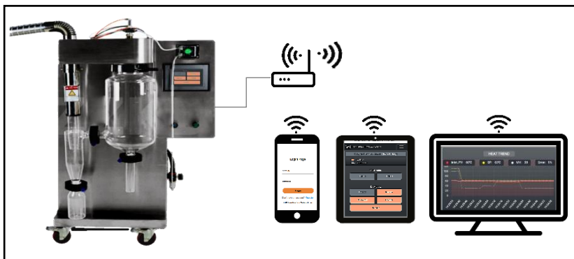
Figure 2. Spray Dryer and Web-Based SCADA
