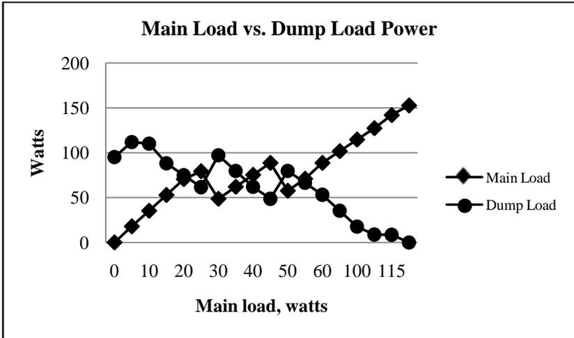
Figure 27. Characteristic mirror image of the main load vs. dump load power absorption
