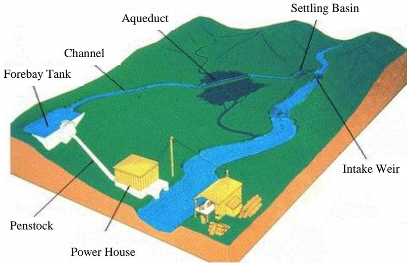
Figure 1. Typical micro-hydro power plant scheme
