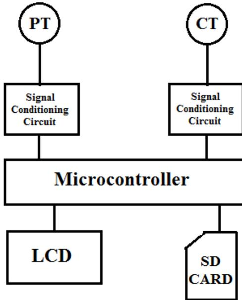
Figure 17. Schematic diagram of the IGMS
