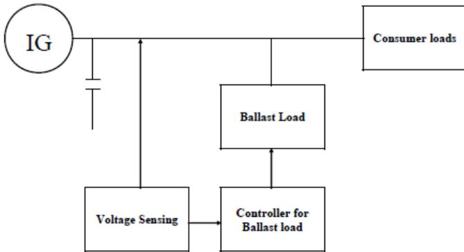
Figure7. Induction generator load control scheme
