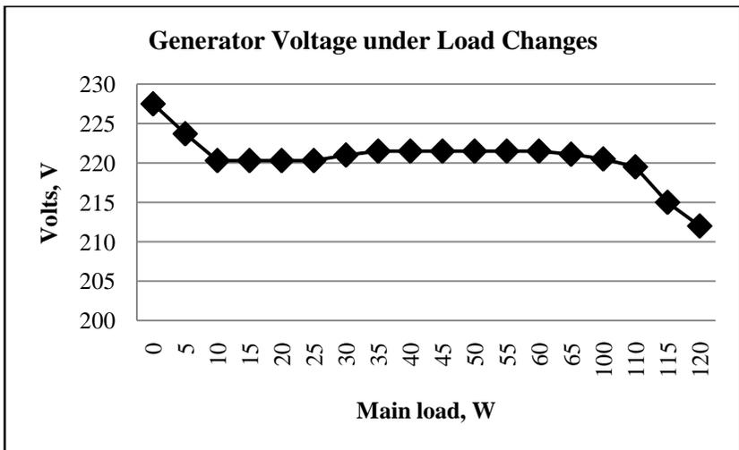
Figure 24. Generated voltage under variable load condition
