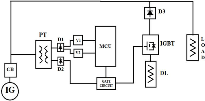
Figure 15. Schematic diagram of the IGCS
