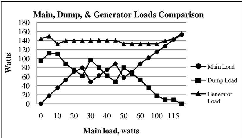
Figure 28. Comparison of the main, dump, and generator loads
