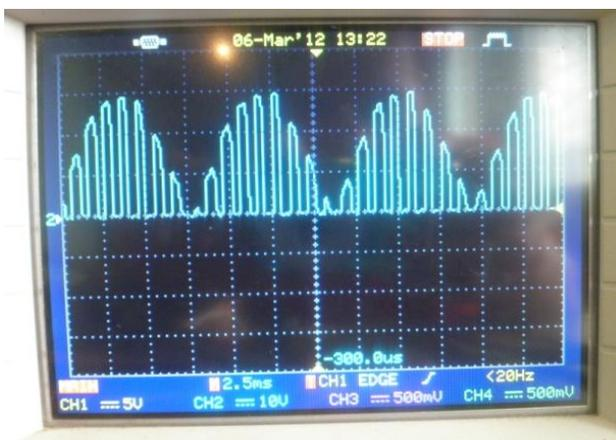
Figure 23. Characteristic output voltage waveform of mark-space ratio controller
