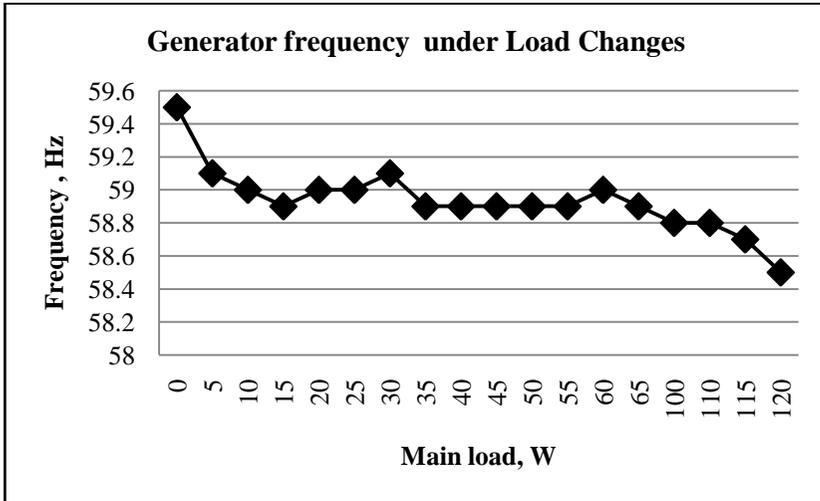
Figure 25. Generator frequency under load changes
