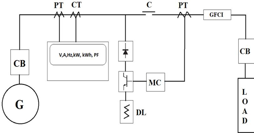
Figure 18. Schematic diagram of the developed IGCMS
