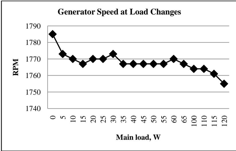
Figure 29. Generator speed at load changes
