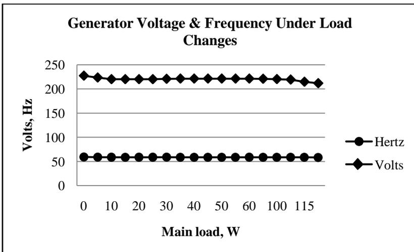
Figure 26. Generator voltage and frequency under varying load conditions
