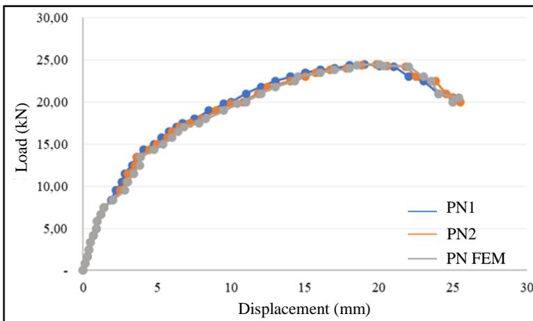
Figure 6. Load versus deflection (PN1, PN2, and PN FEM)
