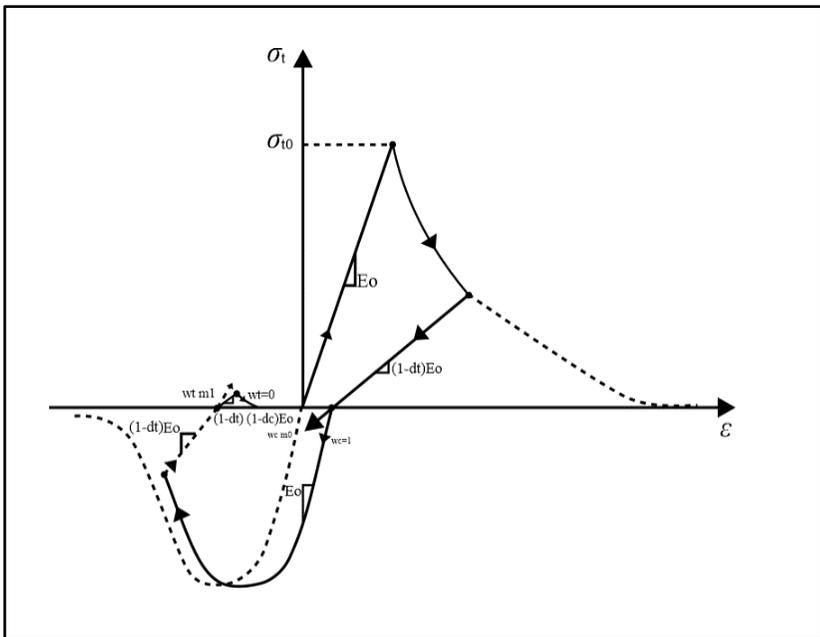
Figure 3. Strength and strain on concrete
