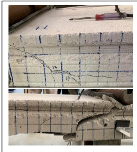
Figure 8. Crack pattern from experimental test
