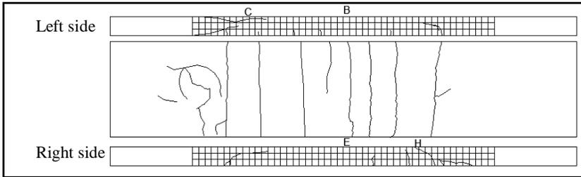
Figure 9. Crack pattern testing for PN1
