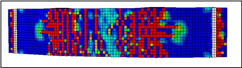
Figure 7. Crack pattern using FEM
