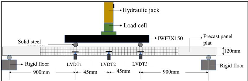
Figure 1. Schematic of flexural testing
