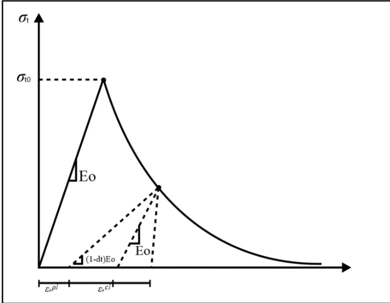
Figure 4. Tensile model on FEM
