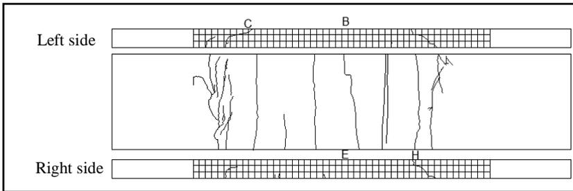
Figure 10. Crack pattern testing for PN2
