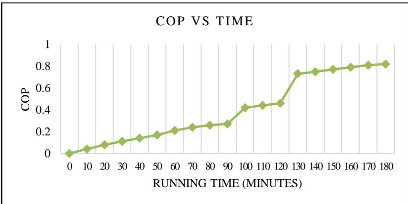
Figure 8. COP vs Time graph of experimental result
