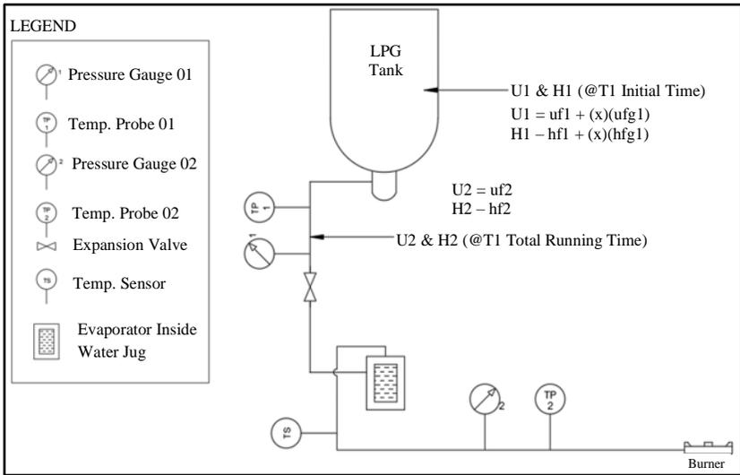
Figure 5. Schematic Diagram of LPG Refrigeration System
