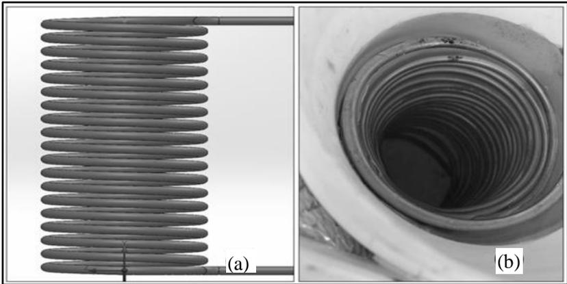
Figure 2. 3D drawing of a cylindrically coiled Copper Tube (a); Actual Copper Tube coiled inside the Evaporator Chamber (b)
