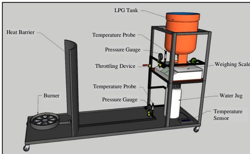
Figure 1. LPG Refrigeration Set-Up with labeled parts
