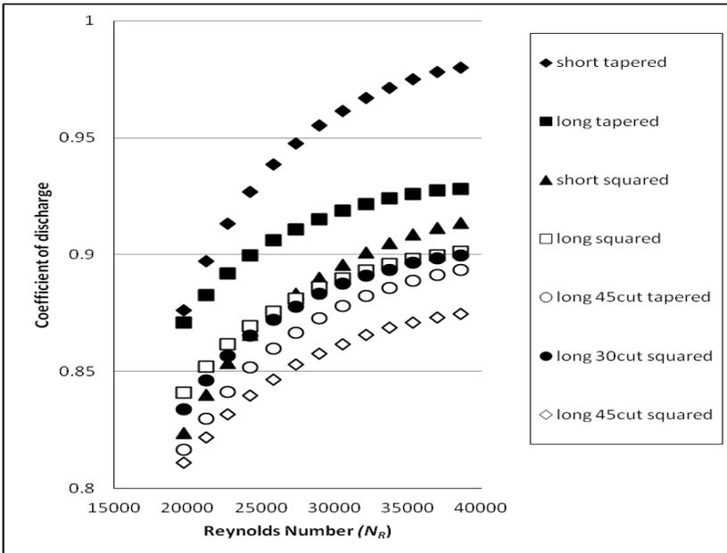
(b) Coefficient of discharge,  $C_d$  vs. Reynolds number,  $N_R$
