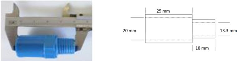
Figure 1. 20 mm UPVC pipe male adapter (*Neltex brand*)
