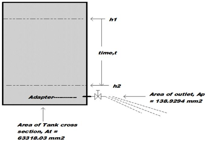
Figure 3. Open tank experiment model
