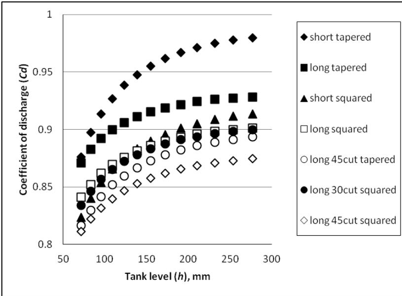
(a) Coefficient of discharge,  $C_d$  vs. head,  $h$
