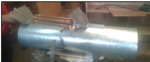
Figure 6. Fabricated heat exchanger assembly, baffles, serpentine coil housing
