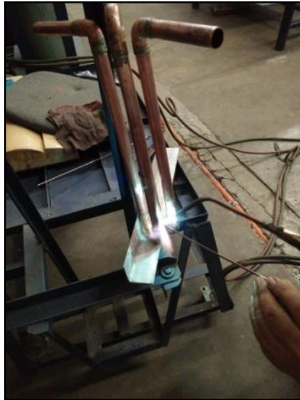
Figure 5. Fabrication of serpentine copper tubing
