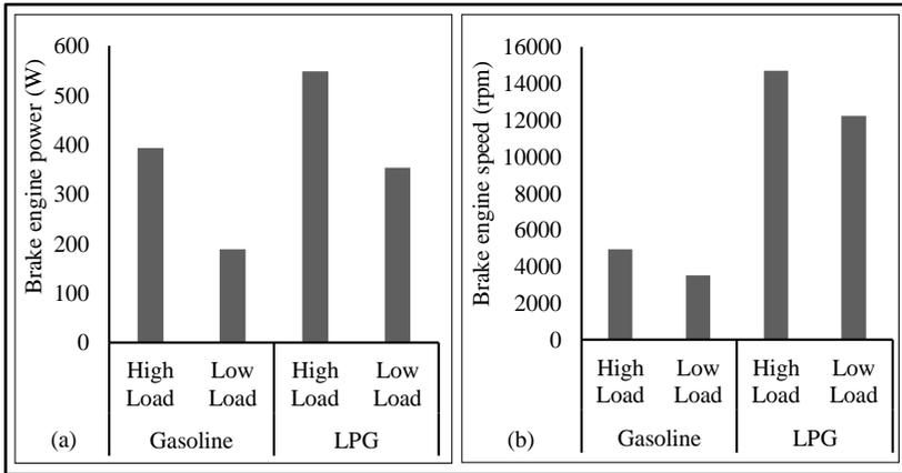
Figure 5. Brake engine power (a) and speed (b) of benchmark fuels
