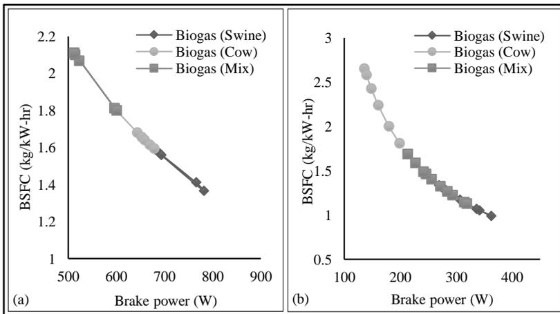
Figure 11. High (a) and low (b) load throttle BSFC of various biogas fuels
