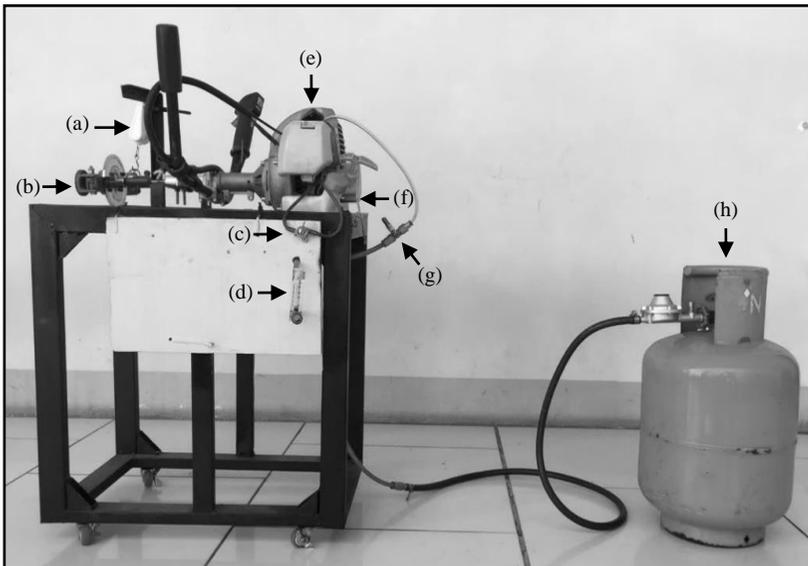
Figure 4. Actual experimental set-up of two-stroke engine fueled by LPG: weighing scale (a), brake dynamometer (b), fuel petcock (c), gas flowmeter (d), engine (e), fuel tank (f), gate valve (g) and LPG (h)
