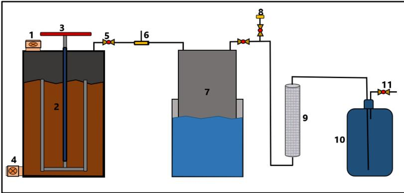
1 – manure inlet; 2 – digester tank; 3 – stirring rod; 4 – digestate outlet; 5 – gate valve; 6 – pressure and temperature sensor; 7 – floating drum; 8 – outlet for testing methane - gas analyzer; 9 – H<sub>2</sub>S removal; 10 – CO<sub>2</sub> water scrubbing removal; 11 – outlet for testing purified biogas - gas analyzer
