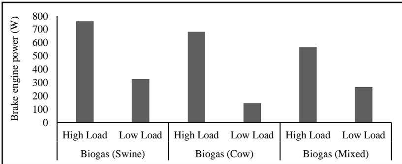
Figure 6. Brake engine power of various biogas fuels
