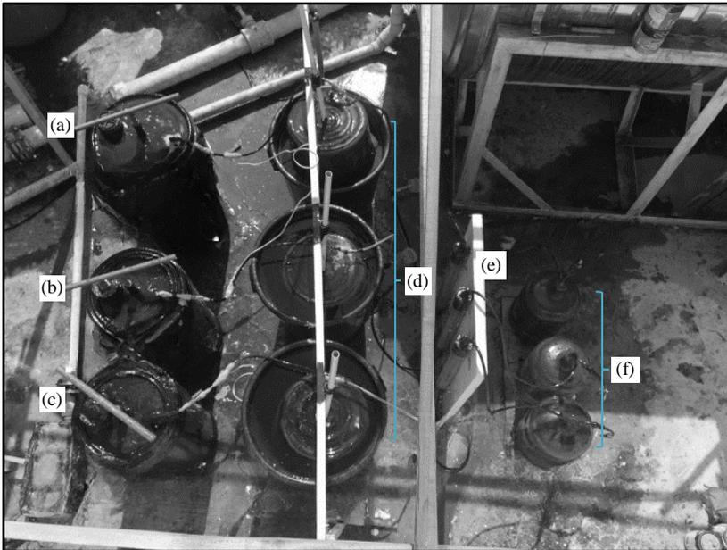
Figure 2. Actual experimental set-up of biogas production: swine-cow manure digester tank (a); cow manure digester tank (b); swine manure digester tank (c); floating drums (d); H<sub>2</sub>S scrubbers (e); CO<sub>2</sub> water (f)
