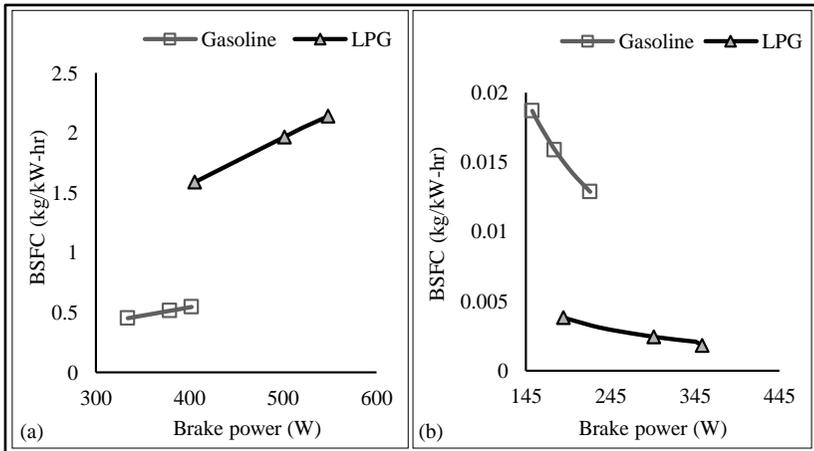
Figure 10. High (a) and low (b) load throttle BSFC of benchmark fuels
