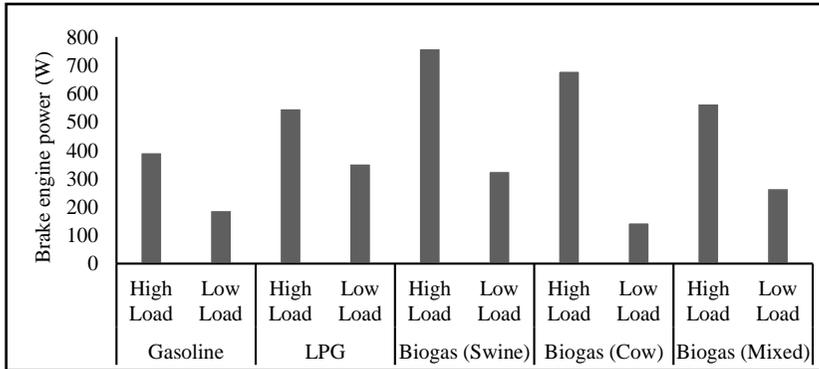
Figure 8. Comparison of brake engine power
