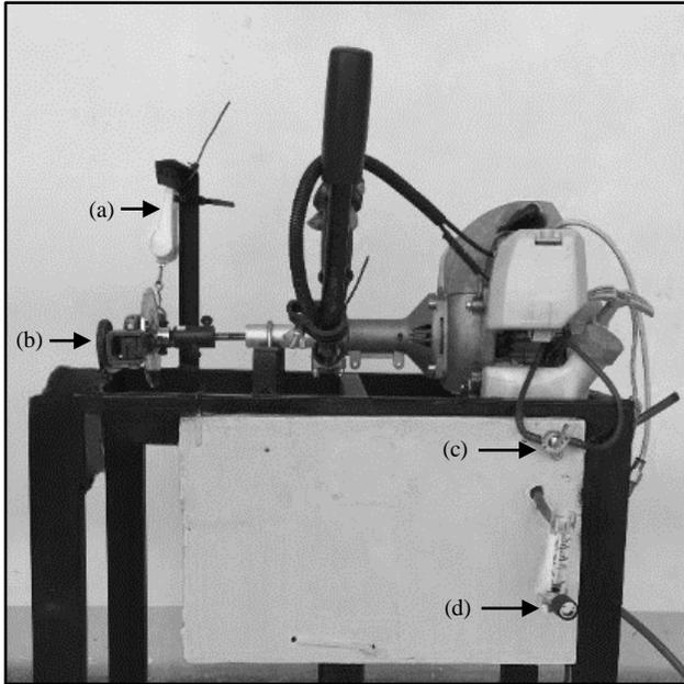
Figure 3. Actual set-up of the two-stroke SI engine: weighing scale (a), brake dynamometer (b), fuel petcock (c) and gas flowmeter (d)
