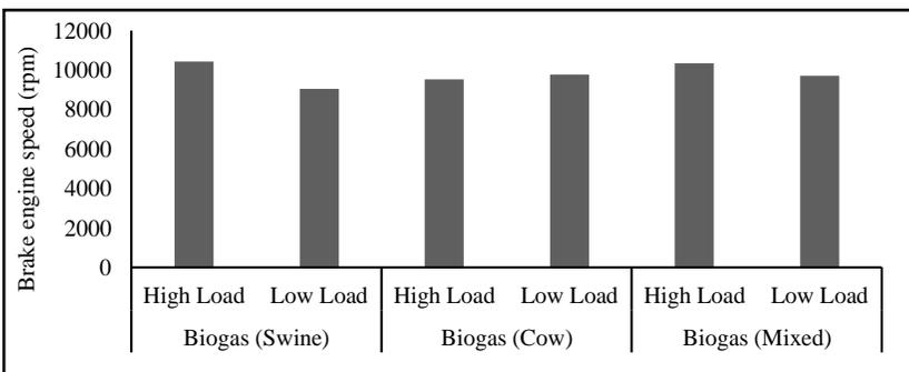
Figure 7. Brake engine speed of various biogas fuels
